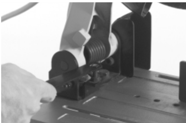
Figure 4 – Adjusting Downstop Screw For Optimum Cut-Off Wheel Height
