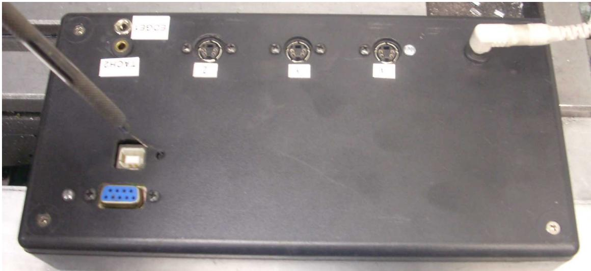
3.  While holding down the button, connect power to the DRO.
