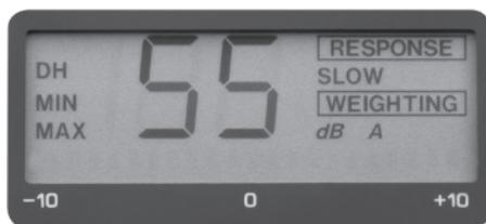
2. Press (or press and hold) **MAX** or **MIN** to set a period from 1 to 199 seconds; position the meter for the measurement.
