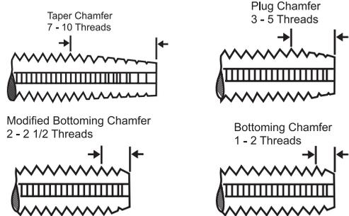
**Taper (7-10 Threads)** - Also known as a starter tap, a taper tap has the longest standard chamfer and requires less tapping torque.
