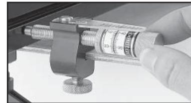
To use it, you set the fence by conventional means, make a test cut, measure the cut error and then use the micrometre to adjust exactly to the finished dimension. This can be done by using the provided fractional/decimal chart (shown on the back page), but a dial caliper is the most convenient tool for the process.
