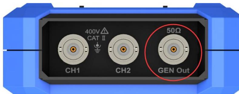
图 6-1: Generator Output Ports
