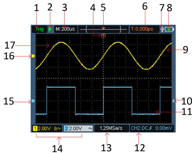
Figure 5: Oscilloscope Interface
