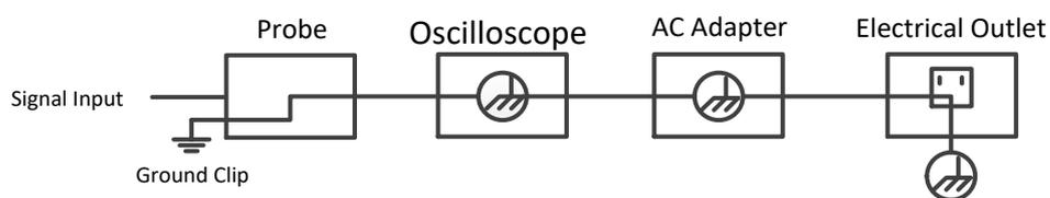
Schematic diagram of internal ground connection when oscilloscope is connected with computer through the port:
