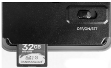
Figure 7: Inserting the SD Card
